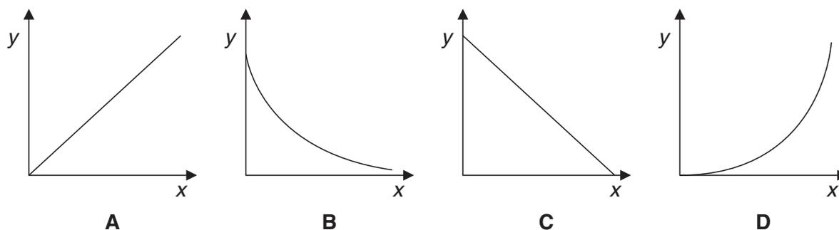
(a) Which graph shows the variation of the **charge** on a capacitor ( $y$ ) against **potential difference** ( $x$ )?
